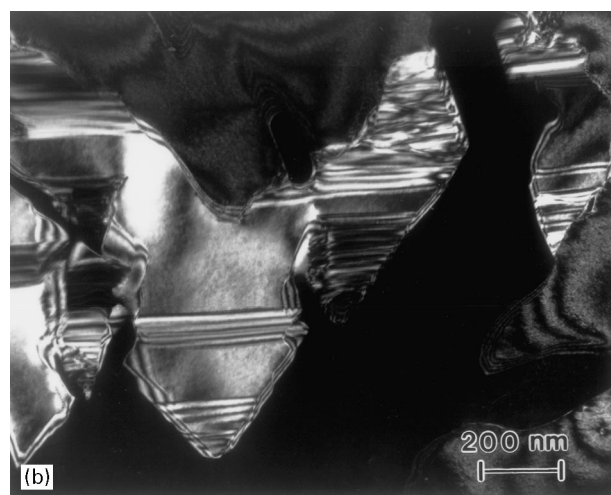
Figure 8 Precipitation of Ni_3Ti in the NiTi substrate adjacent to the bond-line of a sample held for 1 h at 1150 °C: (a) BF micrograph (a = L1_2 type Ni_3Ti , b = D0_{24} type Ni_3Ti , c = \alpha -Cr); (b) DF micrograph ( D0_{24} type Ni_3Ti light, B2 type \beta -NiTi dark, g = (0004)_{Ni_3Ti} ).
