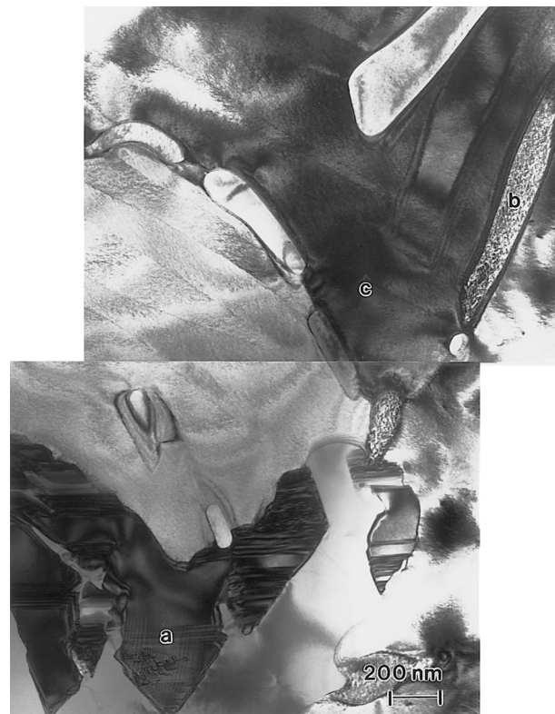
Figure 7 BF montage showing the precipitation of \text{D0}_{24} type \text{Ni}_3\text{Ti} (a) and \alpha -Cr (b) in a B2 matrix (c) containing R-phase precipitates. The figure shows the NiTi substrate adjacent to the bond-line of a chromium-doped sample held for 1 h at 1150^\circ\text{C} .
