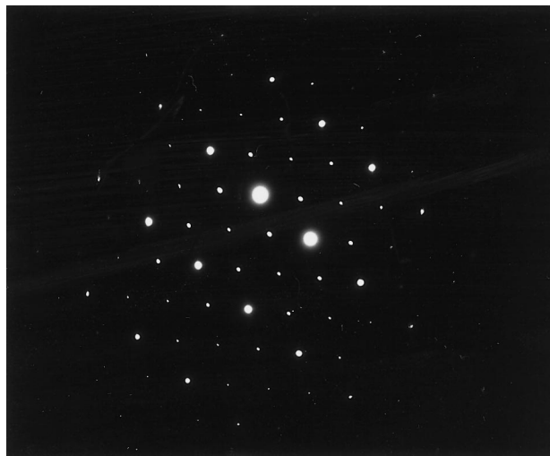
Figure 6 SADP ( B = [110]_{\beta'} ) showing L2_1 type \beta' formed at the joint centre-line of a bond held for 1 h at 1150^\circ\text{C} .
